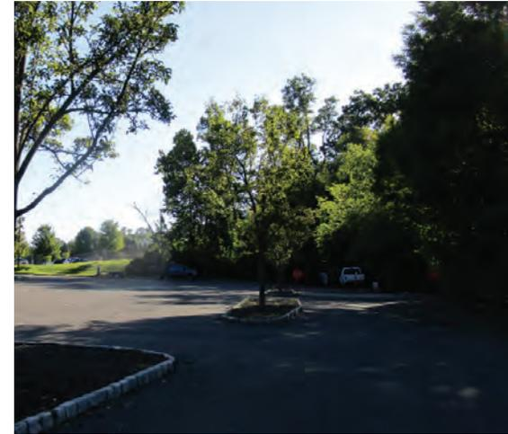
Two sections of parking spaces can be converted to pervious pavement to capture and infiltrate parking lot runoff. Sections of turfgrass adjacent to the parking lot can be converted to rain gardens to capture, treat, and infiltrate parking lot runoff. A preliminary soil assessment suggests that more soil testing would be required before determining the soil's suitability for green infrastructure.
